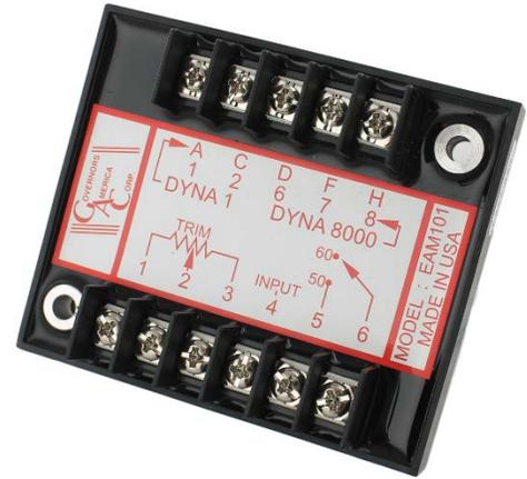
The second terminal block on the EAM101 offers 6 terminals and accepts connections from an external speed trim pot, GAC PIN TP501 or TP503, and signals from the GAC Load Sharing Module, Auto Synchronizer and 50/60 Hz switch.
