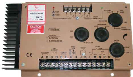
The electronic ESD5300 Series speed control delivers a quick and precise response to transient load changes. When coupled with a proportional electric actuator and a magnetic speed sensor, the ESD will control a wide variety of engines operating in an isochronous, variable, or droop mode. Armed with high quality components, the ruggedly designed ESD will endure the harshness of any industrial engine environment.
