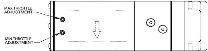
**NOTE** Max throttle Stop is preset to 65 degrees from factory.
